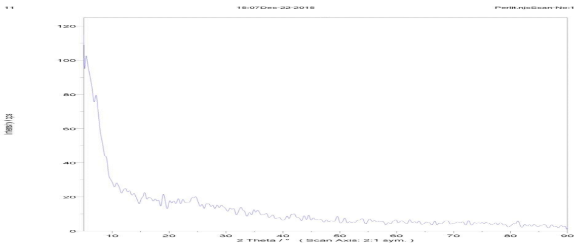
Figure 1. X-ray diffraction pattern of Expanded Nano perlite.
